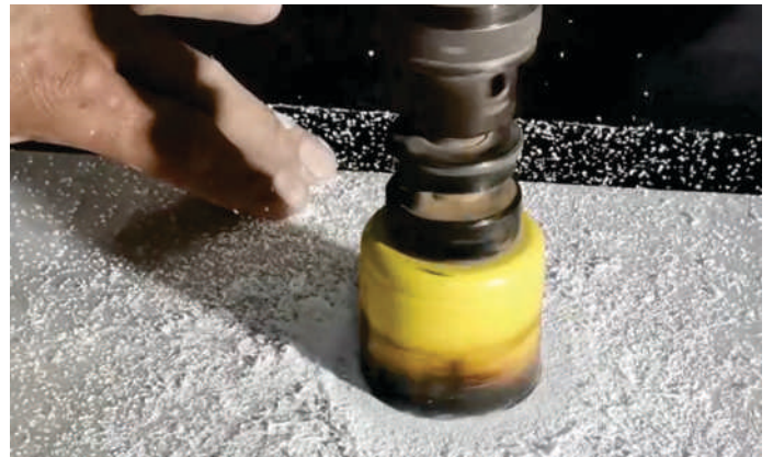
USING A HOLE-SAW ON 8MM LUMOSTONE
